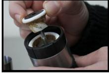
To clean the ceramic grinder burrs, unscrew the white rotary piece and pull the entire internal burr piece straight out, then gently slide the external burr piece out.
